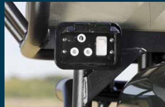
On board Electrical Points
